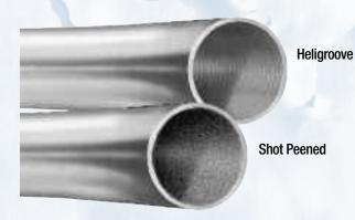
Heli-groove and shot-peened bends and straights reduce angelhair residue in pneumatic/vacuum conveyed plastic pellets.
